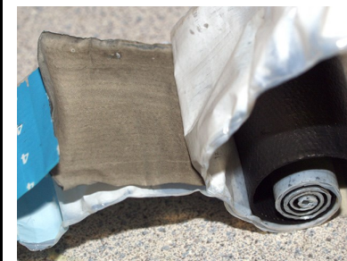
Inside a lithium metal cell
