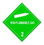
This mark must be a square set at 45 Degree angle, that is diamond shape. The line forming this diamond shape must be 2 mm and the size must be  $100 \times 100 \text{ mm}$
