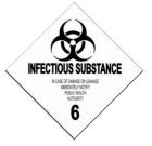
This mark must be a square set at 45 Degree angle, that is diamond shape. The line forming this diamond shape must be 2 mm and the size must be  $100 \times 100 \text{ mm}$
