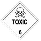
This mark must be a square set at 45 Degree angle, that is diamond shape. The line forming this diamond shape must be 2 mm and the standard size must be 100 x 100 mm
